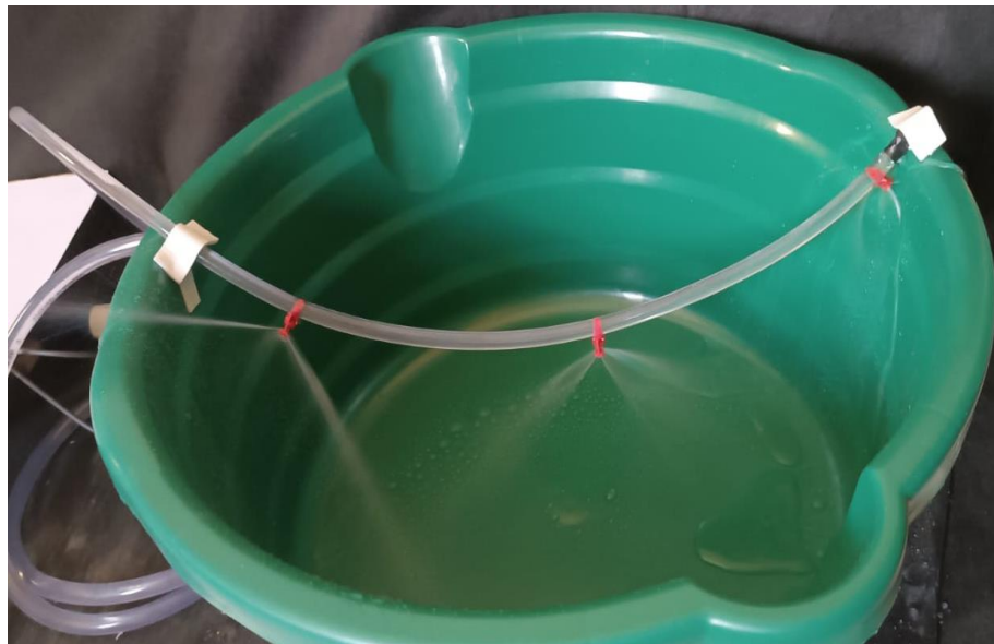
FIGURE 02: Prototype irrigation system using micro-sprinklers connected to a hose.
