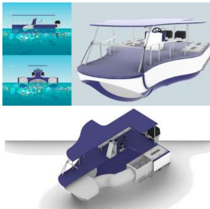
FIGURE 08: Boat for collecting surface waste in coastal waters in side view, front view, perspective view and perspective view.
